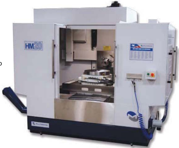
Pictured above: HM20 Linear roller ways, 24 pocket retractable arm ATC
