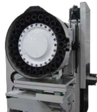
Pictured above: Retractable tool changer Removes ATC from work envelope
